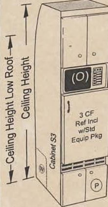
CABINET S3 If desired, two drawers can locate in bottom. If no microwave space becomes storage.
