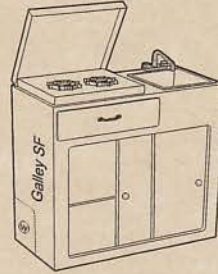
GALLEY SF 18" depth of galley E and F allows for walk space when located across from gauchio when bed is made up. Sliding or hinged doors.
